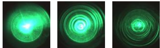
(a)滑らか(Ra0.05) (b)少し粗い(Ra0.36) (c)粗い(Ra1.36)
