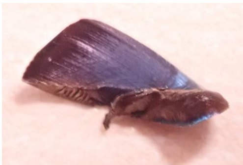
Fig.7 Chip of work piece(pass1)
