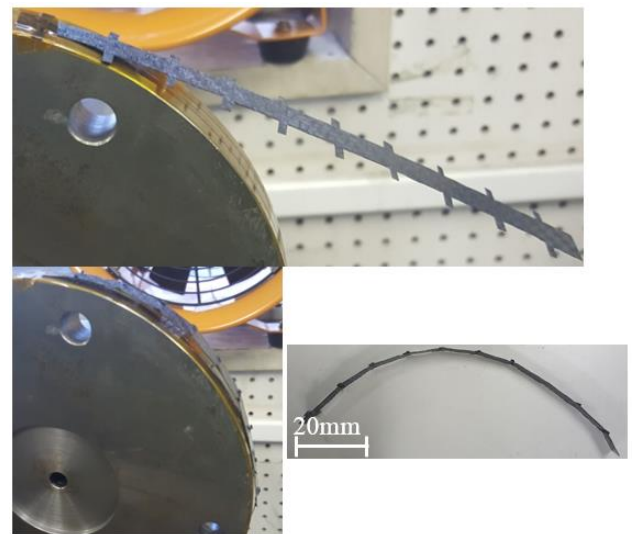
Fig.6 Incremental bending by electric heating
