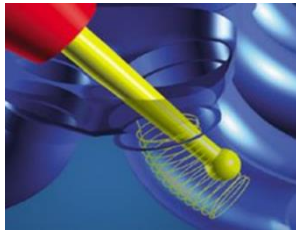
Fig.1 Spiral path for tube machining [1]
